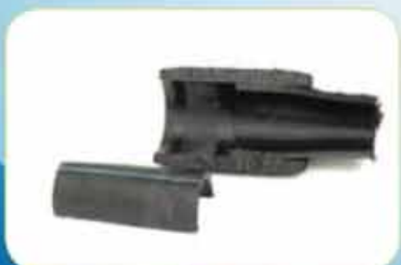
Lack of Scraping
