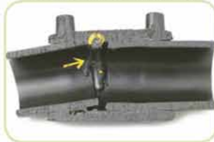
Off-Centering of the Pipe on the Left Side
