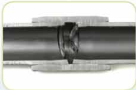
Pipe Boring Before Cooling
