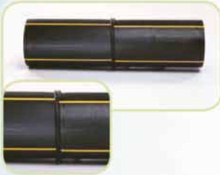
Irregular Welding Bead
