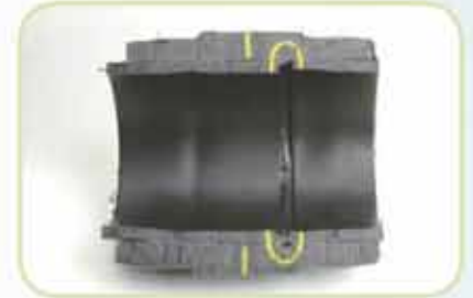
Wrong Centering of the Pipes
