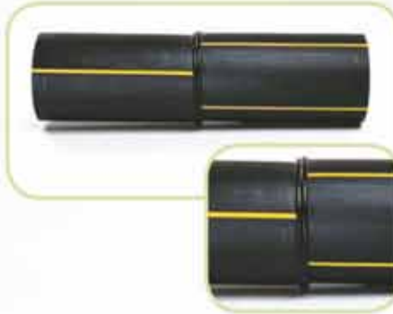
Butt fusion Off-Centering of the Elements
